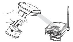
Two quick beeps followed by clicking, then a single beep indicates a "good" association. The scanner is in communication with the base. If the scanner clicks for 30 seconds and signals an error (triple beep), it has not associated with the base.
